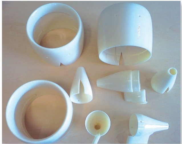
RedEye’s FDM additive manufacturing services were engaged to produce engine nacelle parts for the wind tunnel model. Image Courtesy of Aurora Flight Sciences.
