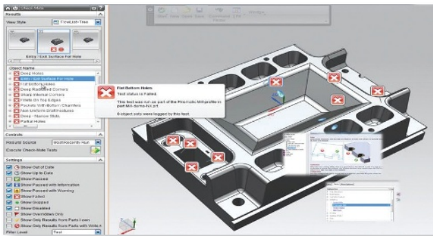
The DFM module automatically checks and identifies potential production problems based on CAD geometry.
