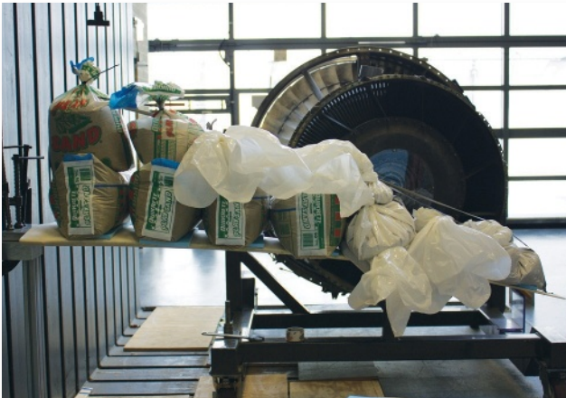
In one test, an FDM wing with an aluminum skeleton was mounted upside down and loaded with 340 pounds to simulate a 300% loading of maximum lift force in the tunnel, resulting in a wing tip deflection of 8 inches. Image Courtesy of Aurora Flight Sciences.
